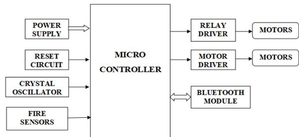
Fig-1: Architecture of Microcontroller
