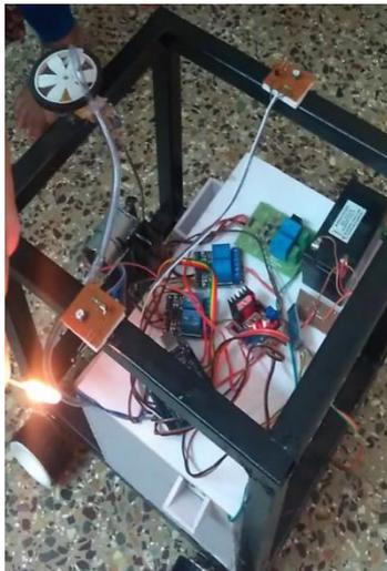
Fig-11: Fire detected at Left end
